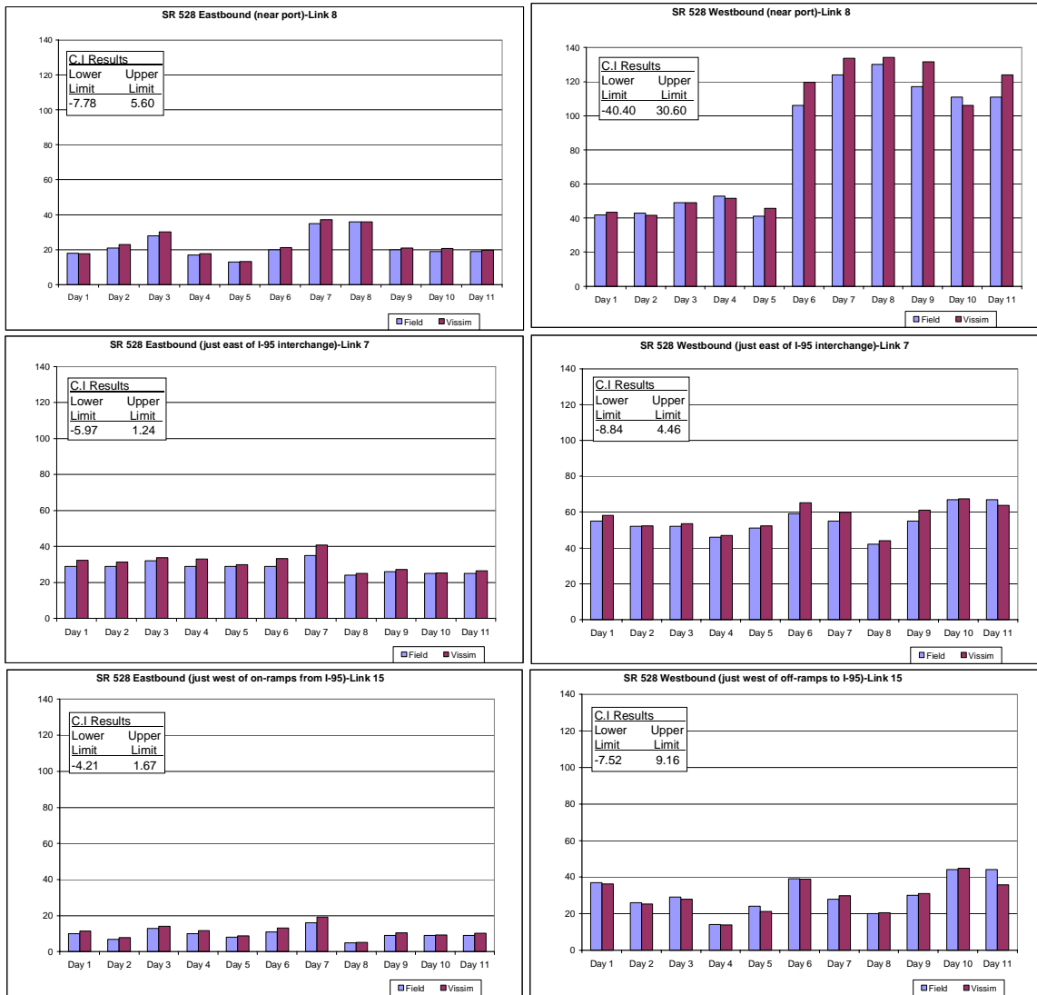
Figure 3: Port Canaveral Field and VISSIM Truck Volume Validation Results
